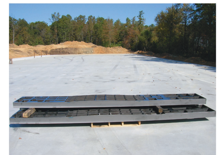
Gray Iron (CL 30) Bridge for Textile Machinery - 3820 pounds.
