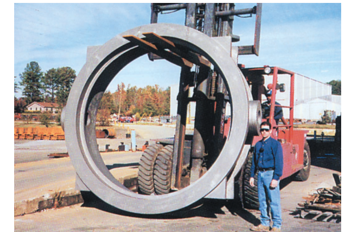
Gray Iron 120" Butterfly Valve Body (A126 Class B) - 22,240 pounds.
