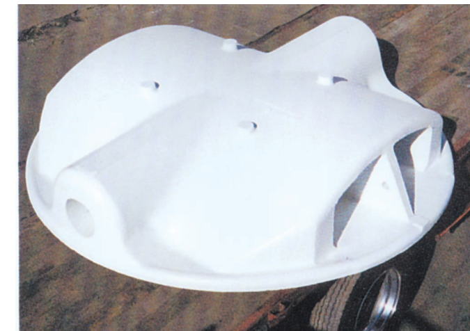
Ductile Iron 120" Butterfly Valve Disc (65/45/12) - 27,000 pounds.
