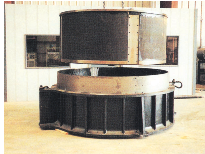
Gray Iron Cylindrical Valve Body and Cylinder for the Panama Canal (A126 Class B) - 7200 pounds each.
