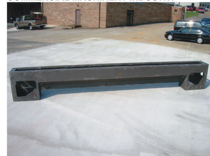
Gray Iron (CL 30) Housing for Carpet Manufacturing Machine - 11,880 pounds.
