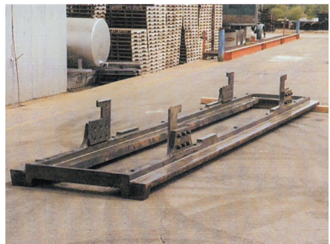
Ductile Iron 6 Meter Coke Oven Door Jamb (65/45/12), machined and assembled - 8840 pounds.
